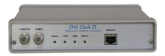
The core of the CNS Clock II is a GPS receiver module. The standard version of the CNS Clock II features the best available receiver, the Motorola Oncore M12+(T) or i-Lotus M12M.
