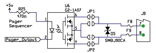
**Interface:** The interface is designed to connect directly to a variety of pager terminals by using the terminal's "Busy" line. This includes thee Zetron 2200, Kantronics Model 2000, Motorola Unipage M15 Paging Terminal and the GlenAyre GL3000.
